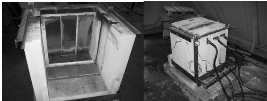
Figure 3 To the left: View inside the test equipment showing the electric heated foil. The specimen is placed just in front of the foil. To the right: Outside view of the experimental stand. Three phase electric supply is connected.
