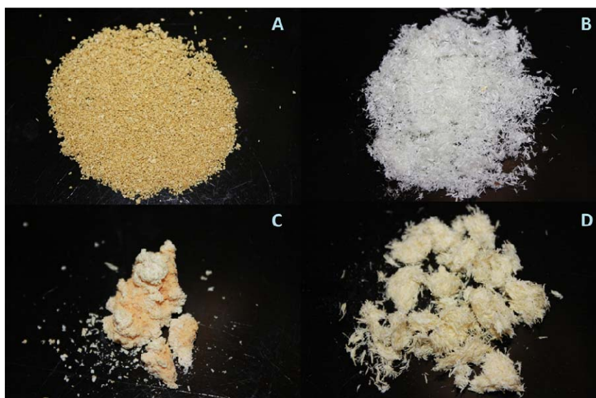
Figure 2: Cellulose residues from hazelnut shells (A), wheat straw (B), orange peels (C) and brewer's spent grain (D) after lignocellulosic fractionation.
