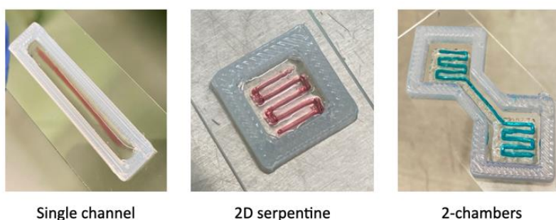
Figure 2. Bioprinted structures. The structures are contained in a 3D bioprinted silicone mold (SE-1700) to aid in needle placement at the ends of the channel.
