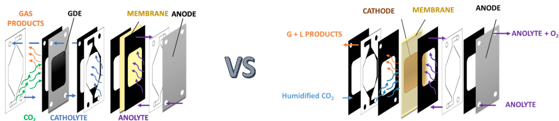
Figure 1. Schematic layouts of the GDE (left) and MEA (right) configurations.
