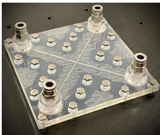
Figure 1. Picture of the fabricated PMMA device for the experiments.
