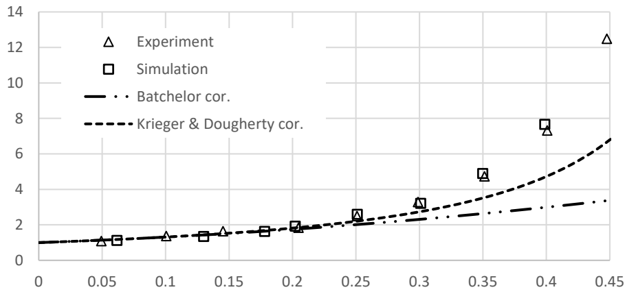
Figure 1: Results of the viscosity study for suspensions made of spherical particles. Trinagles represents experimental data, squares simulation data, dashed line stands for Batchelor's correlation and dashed-dotted line for correlation by Krieger and Dougherty
