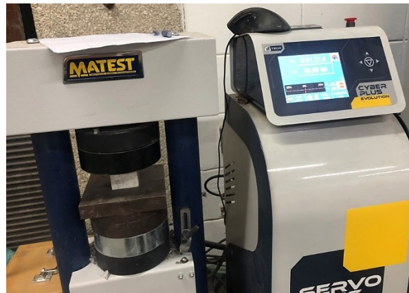
Figure 1. Compression testing of paste samples
