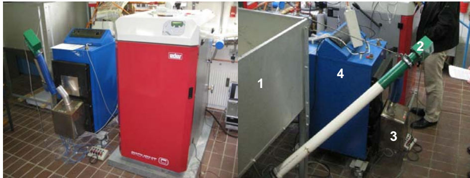
Figure 1: Left: Pellet burner (blue) and wood gas burner (red) in the laboratory of Dezentrale Energiesysteme at the institute for energy technique and motion technique, University of Applied Science, Ulm. Right: Pellet burner with pellet storage and auto feeding system. Legend: 1: Storage for wood pellets, 2: Electrical auto feeding system, 3: Pellet burner with control unit and housing, 4: Burner, adapted for experimental use, originally a simple wood burner.
