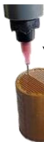
Figure 1 3D-Printing of the microstructured reactor by paste extrusion of \text{Fe}_{15}\text{Co}_{15}@/\text{Al}_2\text{O}_3
