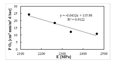
Figure 4: Relation between the experimental values of O₂ Permeability coefficient and the Elastic modulus.
