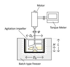
Figure 2: Experimental apparatus consisting of batch type freezer, motor agitation impeller and torque meter
