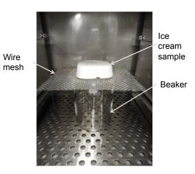
Figure 3: Experimental setup for melting test
