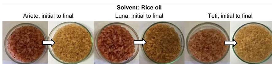
Figure 8: Photos of the colour variations in rice kernels varieties (day 0 to day 63) using rice bran oil as solvent.
