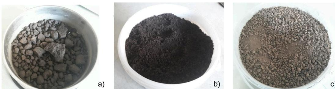
Figure 1: a) Non-passing fraction of the 5 mm sieve, b) sieved hydrocarbons polluted soil, c) depolluted soil
