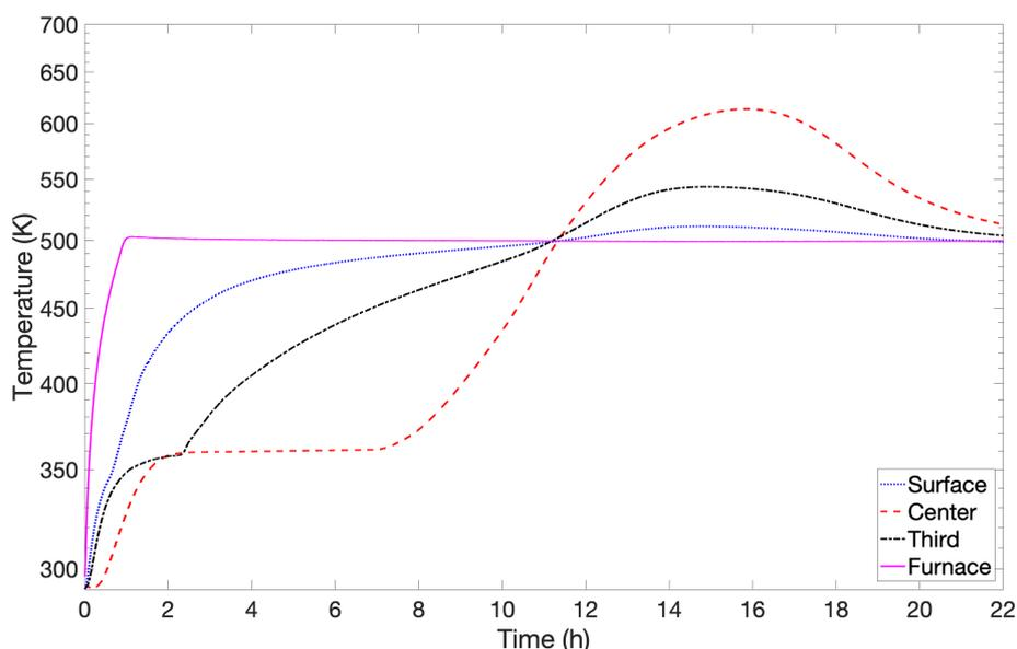
Figure 2: Example of a self-heating test on a soil polluted by hydrocarbons in a 8000 cm<sup>3</sup> basket at 230 °C
