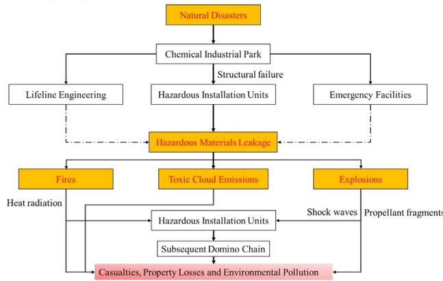
Figure 1: The general system dynamic response process
