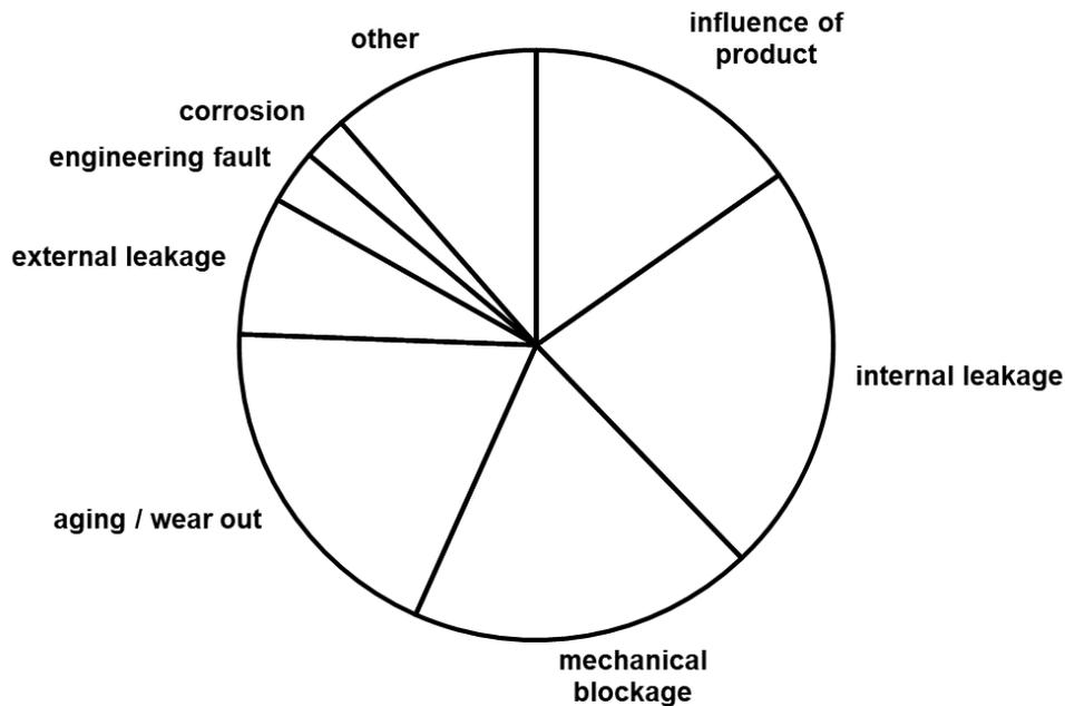
Figure 1: Failure modes for the defective components "actuator" and "final element" (valves) for the years 2017-2019
