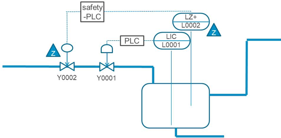
Figure 2: Typical safety function, safeguarding a vessel against overfilling (NAMUR WG Practice Paper, 2021)
