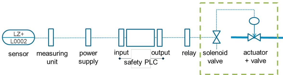
Figure 3: Signal path of the safety function and "extended valve" (NAMUR WG Practice Paper, 2021)
