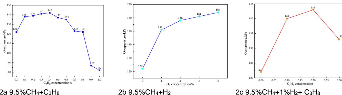
Figure 2: multicomponent gas explosion pressure under different working conditions
