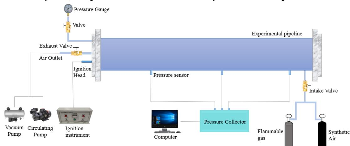
Figure 1: Schematic of gas explosion experiment device
