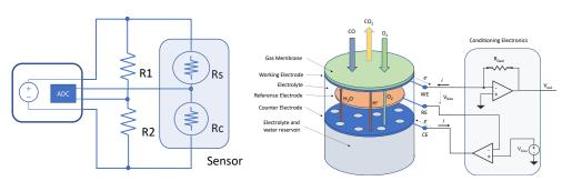
Figure 3 – (left): Conditioning electronics for catalytic sensors. (right): Conditioning electronics for electrochemical sensors.
