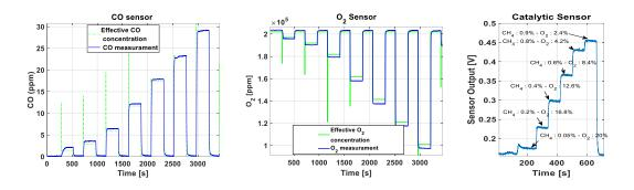
Figure 4 – CO and O<sub>2</sub> electrochemical sensor tests and catalytic sensor test with methane.
