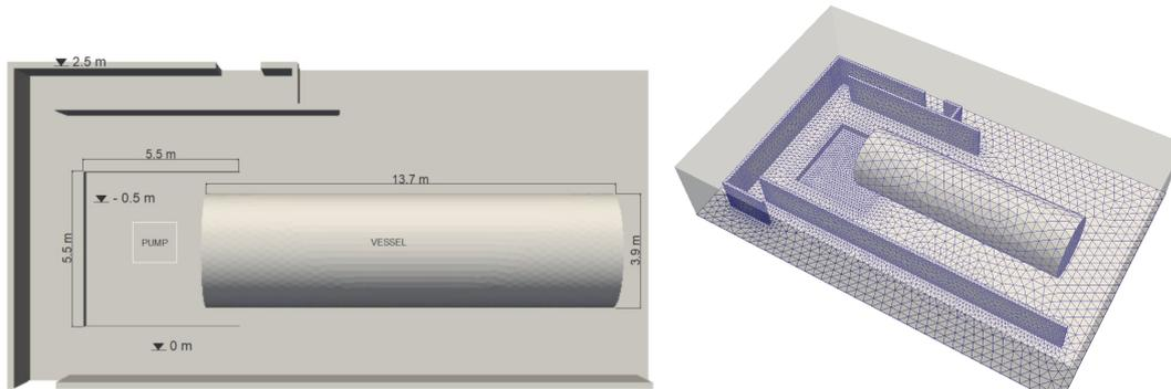
*Figure 1: 3D model of storage area and computational mesh*
