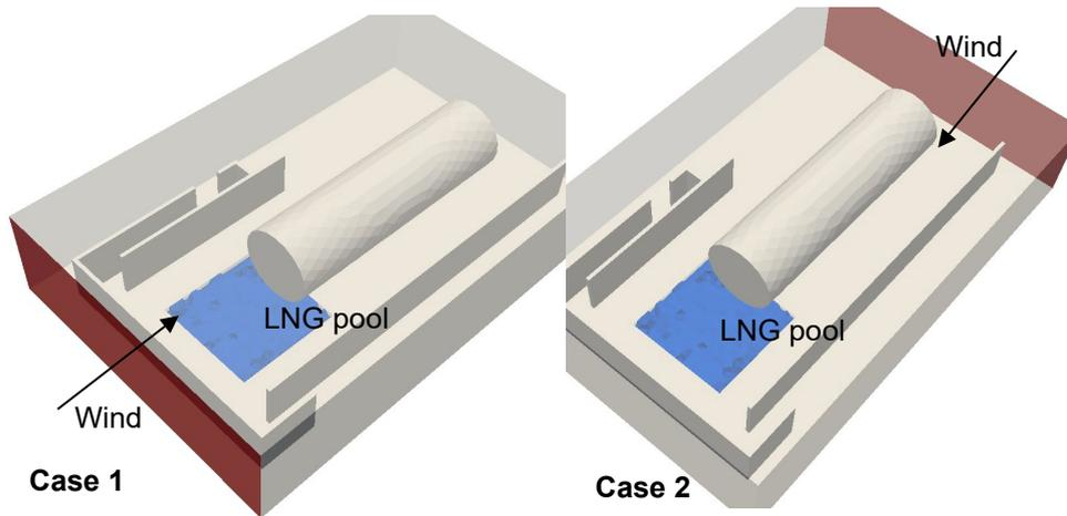
Figure 2: Boundary conditions for Case 1 and Case 2
