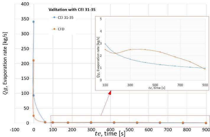
Figure 3: Comparison of results obtained with CEI 31-35 and CFD
