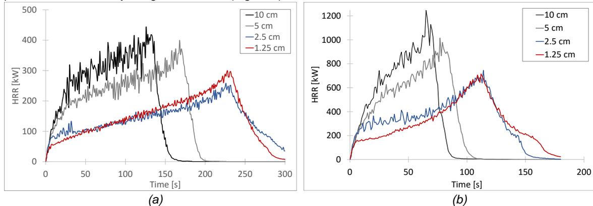
Figure 2: Grid sensitivity analysis for HRR prediction. Square pool fires: (a) 0.3 x 0.3m; (b) 0.5 x 0.5m
