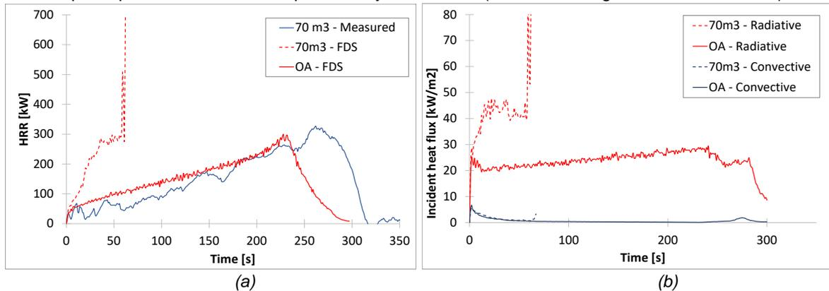
Figure 4: (a) Comparison of measured and predicted HRR for the  $0.3 \times 0.3 \text{ m}$  pool fires in the  $70 \text{ m}^3$  airtight setup and in open atmosphere (OA); (b) Simulated incident heat flux on the pool surface
