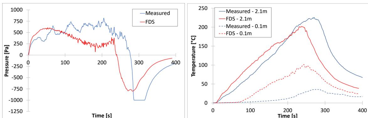
Figure 5: Comparison of measured and predicted fire induced pressure and fire room temperature for the  $0.3 \times 0.3 \text{ m}$  pool fire in the  $70 \text{ m}^3$  airtight setup.
