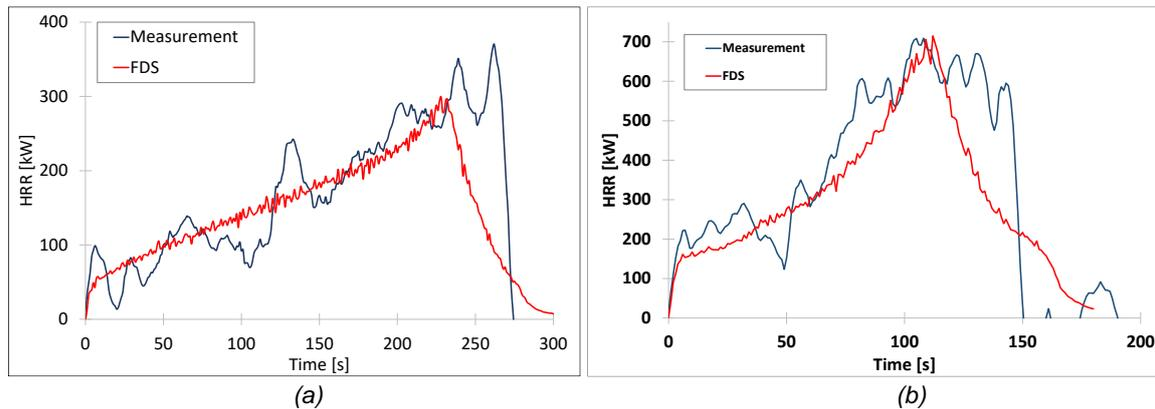
Figure 3: Comparison of measured and predicted HRR. Square pool fires: (a) 0.3 x 0.3m; (b) 0.5 x 0.5m
