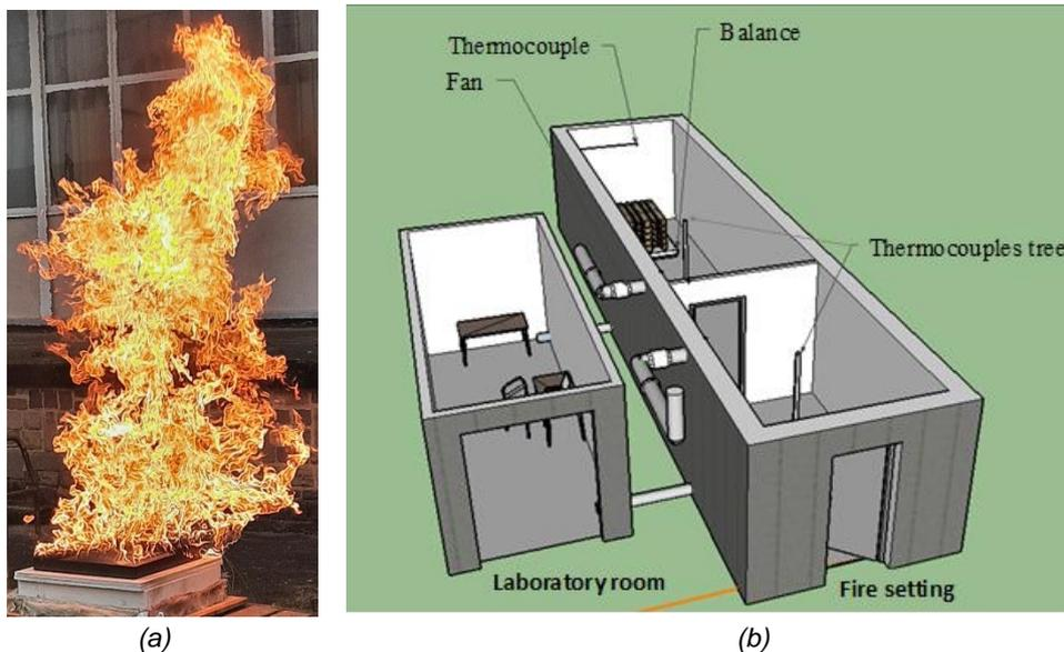
Figure 1: (a) Heptane pool fire in open atmosphere (50cm x 50cm pan); (b) Sketchup of the 70 m<sup>3</sup> airtight setup
