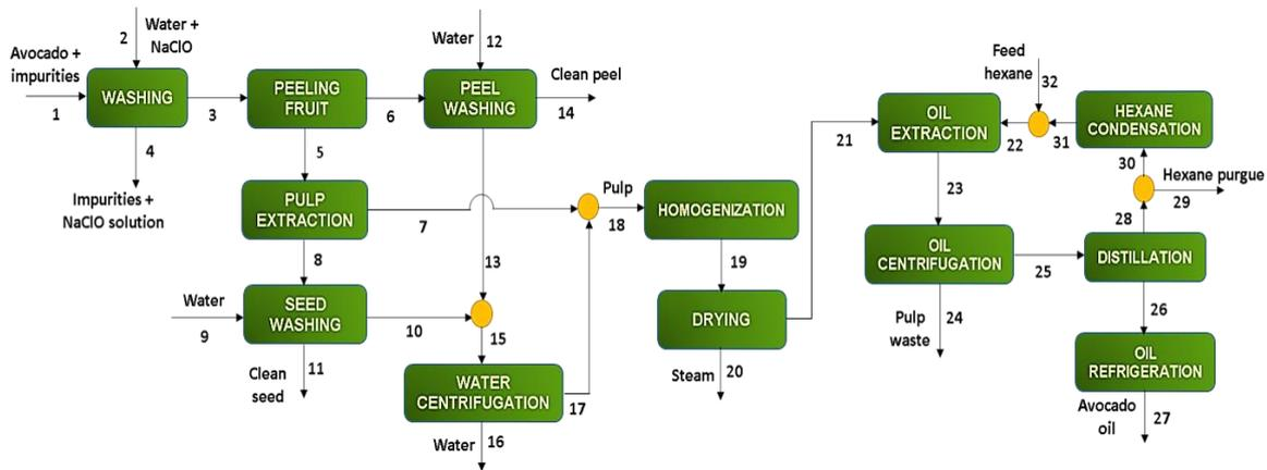
Figure 1: Process flow diagram of avocado oil extraction.
