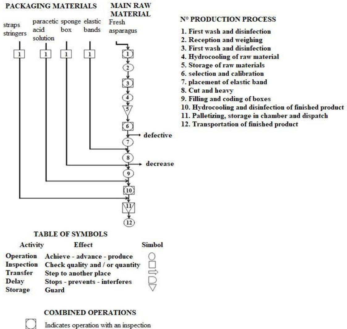
Figure 1 Process diagram of fresh asparagus processing.
