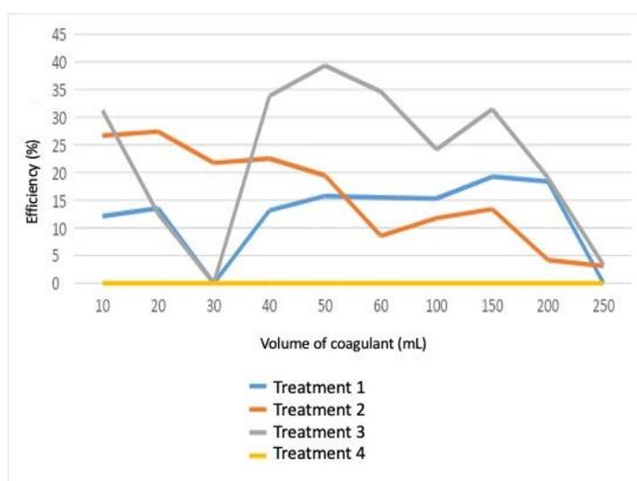
Figure 3 - Color removal efficiency using organic coagulant extracted from *Inga nobilis*.
