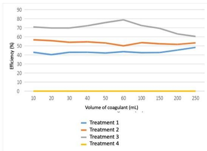
Figure 4 - Turbidity removal efficiency using organic coagulant extracted from *Inga nobilis*.
