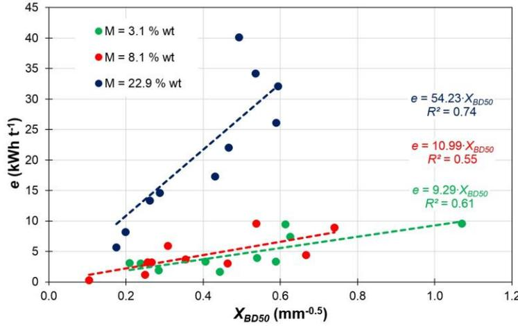
Figure 3: Modelling energy demand on particle size characteristic  $D_{50}$  and moisture  $M$  by Bond theory.
