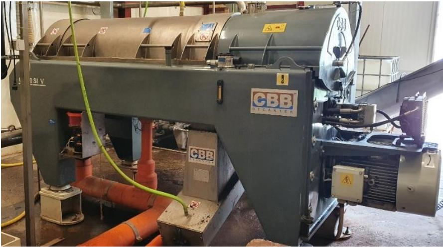
Figure 3: industrial centrifuge at Mezzocorona waste management plant for HTC slurry treatment
