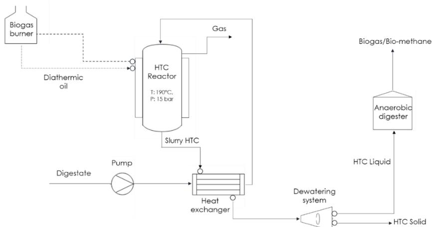
Figure 1: Schematic representation of the continuously operating C700 HTC plant.
