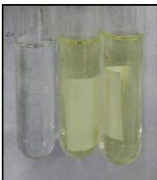
Figure 5: Test tubes showing a mixture of solutions containing heavy metals. Three sample solutions were the first sample is the control solution, and the second and third contain paper strips with latex.
