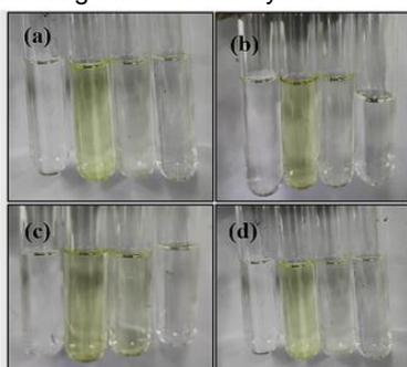
Figure 6: Test tubes showing solutions of (a) Ferrous Ammonium Sulfate, (b) Potassium Dichromate, (c) Cadmium Sulfate, (d) Lead Nitrate with the same concentration (0.5 ppm). The paper strip used was coated with 5 ml latex.
