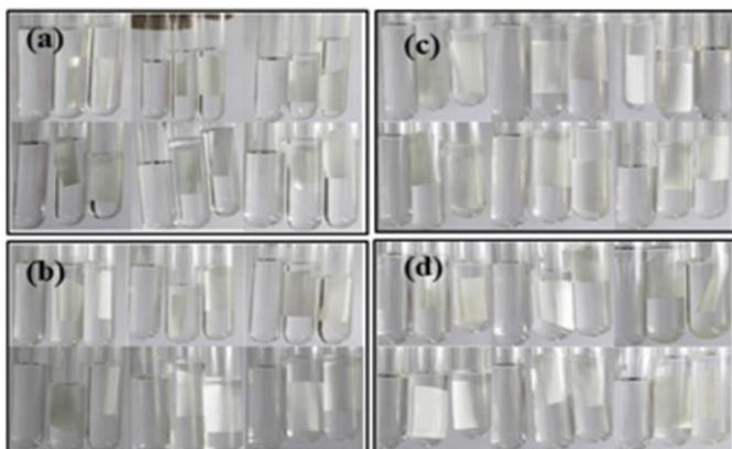
Figure 4: Test tubes showing solutions of (a) Ferrous Ammonium Sulfate (b) Potassium Dichromate (c) Cadmium Sulfate (d) Lead Nitrate with increasing concentrations (0.05, 0.1, 0.25, 0.5, 0.75, 1 ppm) respectively. Paper strips used came from a paper sheet coated with 5 ml of latex. Each test included a control (solution without paper strip) and two replicates for each concentration.
