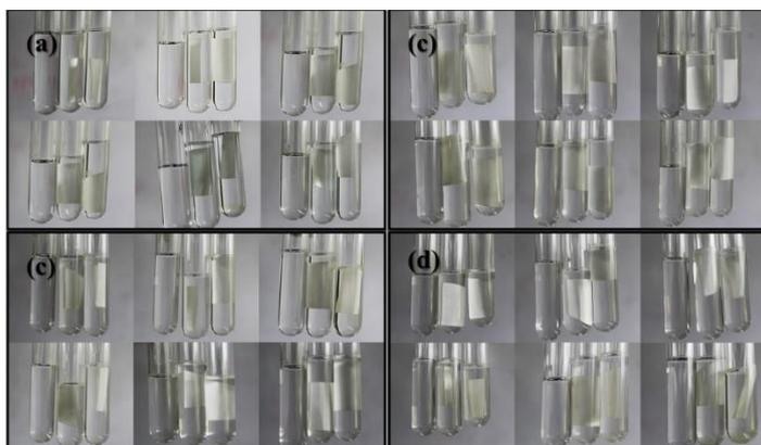
Figure 2: Three samples of each type of solution of Ferrous Ammonium Sulfate, Potassium Dichromate, Cadmium Sulfate, and Lead Nitrate were run. These solutions contain the heavy metals Fe, Cr, Cd, and Pb, respectively, with an increasing concentration of 0.05 ppm to 1.0 ppm. The left-most solution served as the control (no paper strip), while the second and the third samples contained a paper strip coated with kalachuchi latex to detect the presence of heavy metal ions present in each solution.
