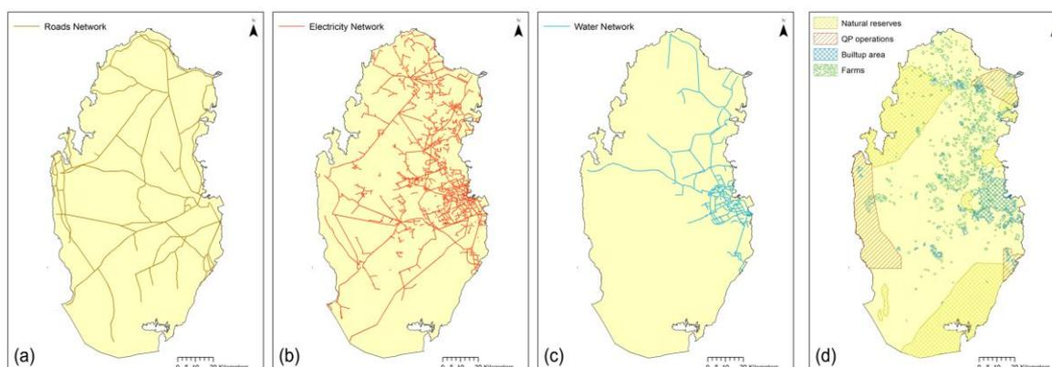
Figure 2: Key infrastructural facilities in Qatar including a) roads network, b) electricity network, c) water network, and d) defined restricted areas.
