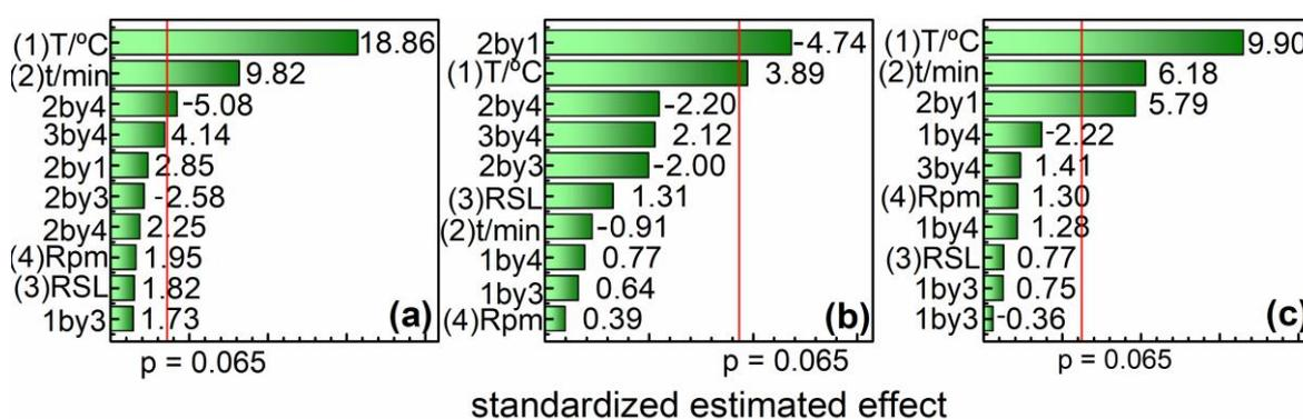
Figure 3: Pareto charts of standard effects for temperature (T), time (t), SLR e agitation (Rpm) in hemicellulose conversion (a), release of xylose (b) and furfural (c) with a significance level of 0.065
