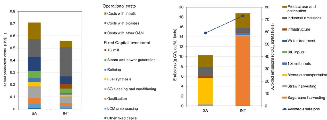
Figure 2 – (a) Biojet fuel production costs breakdown and (b) total emissions and avoided emissions (CO<sub>2</sub> eq)
