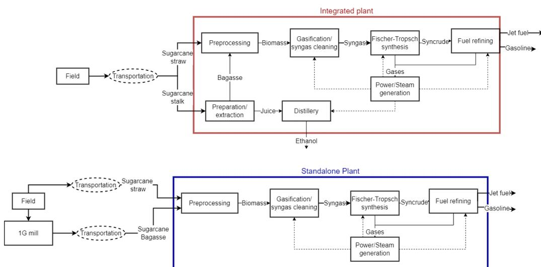
Figure 1 – Simplified process flowchart for the integrated and standalone configurations
