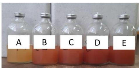
Figure 5: Selenium suspensions for various concentrations 0 mg/L (A), 15 mg/L (B), 30 mg/L (C), 60 mg/L (D) and 120 mg/L (E) of Na<sub>2</sub>SeO<sub>3</sub> in 50 mL medium culture after 24 h.
