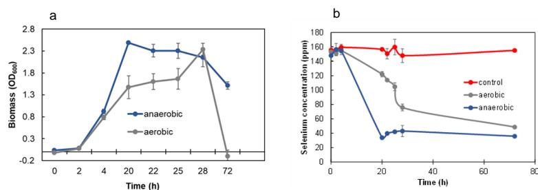
Figure 1: Time course of a) biomass production b) selenite reduction under aerobic and anaerobic conditions.
