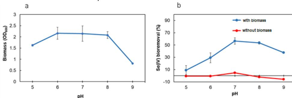
Figure 3: Effect of initial pH (5-9) on a) bacterial growth b) selenite bio-removal after 24 h incubation.
