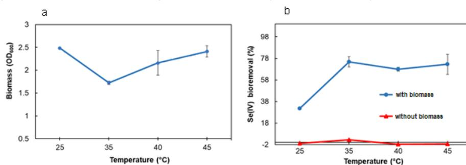
Figure 2: Effect of temperature (25 -45 °C) on a) bacterial growth b) selenite bio-removal after 24 h incubation.
