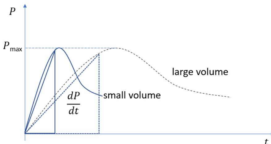
Figure 3. Diagram of pressure vs time showing the difference in rate of pressure and explosion duration for two different volumes; the larger volume is represented by the dashed line.
