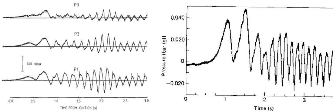
Figure 4. Left: Oscillatory pressure development resulted in the ignition of the upper half of a silo of  $236\text{m}^3$ . The fuel is cornstarch  $600\text{g}/\text{m}^3$  and vented on the roof with  $5,7\text{m}^2$  vents. Right: Pressure vs time measured at  $3\text{m}$  above the bottom of the silo. Figure as seen in Eckhoff (2003), Eckhoff (1988) and Eckhoff (1984).
