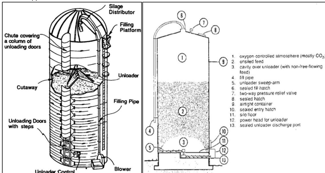
Figure 2. The schematic of a conventional silo (left) and a limiting oxygen silo (right). (Clark et al., 1998)
