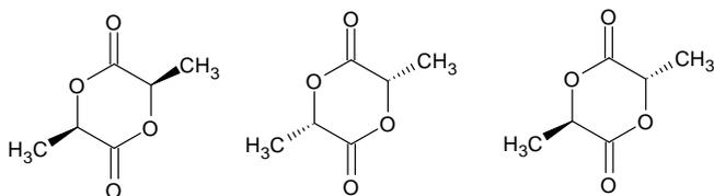
Figure 1: Chemical structure respectively of L-lactide, D-lactide, D, L-lactide, Source: Produced in ChemSketch based on (Groot *et al.*, 2010).
