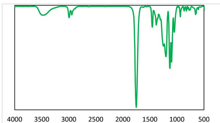
Figure 7: FTIR of L-lactide collected during the experiment.
