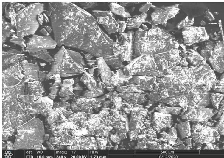
Figure 5: SEM analysis about PLLA obtained
