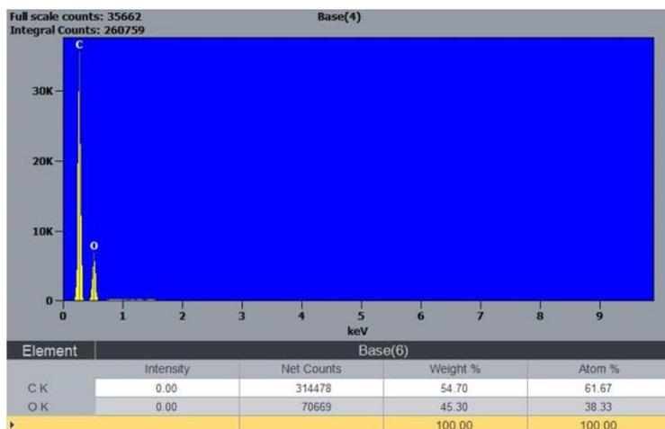
Figure 6: Analysis of the chemical composition of PLLA
