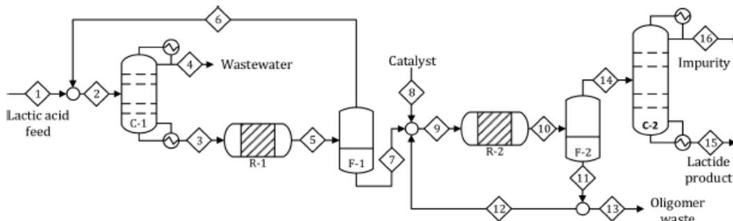
Figure 2: Process flow diagram of L- lactide synthesis process (Heo *et al.*, 2019).
