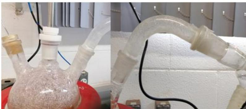
Figure 4: Encrustation obtained in 12 h and 8 h respectively.
