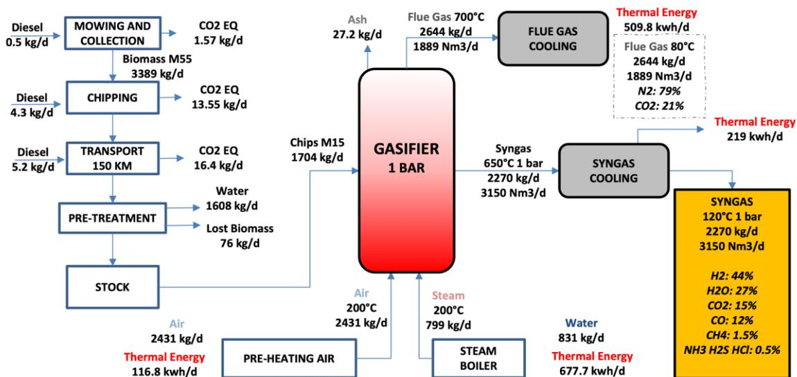
Figure 2 Gasification supply chain. M55 means a humidity percentage of 55% and the syngas composition is given in massif percentage.
