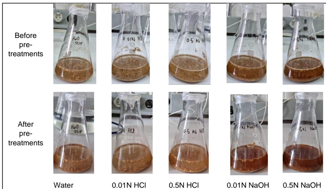
Figure 1: Physical observation of BSG samples before and after different pre-treatments
