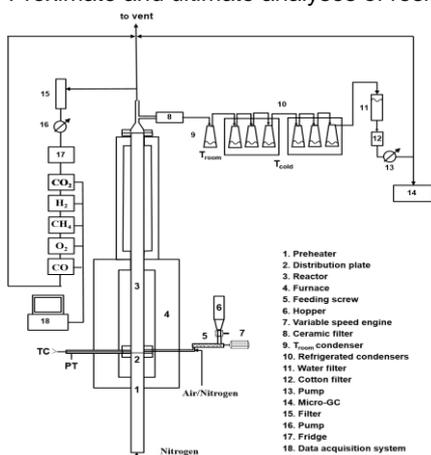
Figure 1: Schematic of the experimental apparatus
