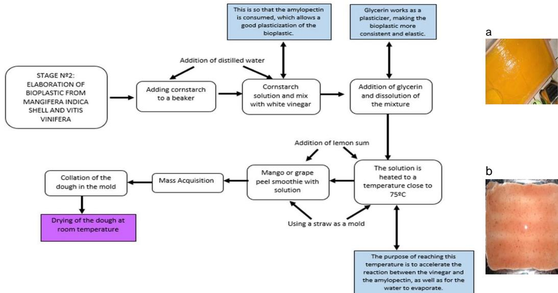
Figure 2: Elaboration of the bioplastic from the shell of *Mangifera indica* and *Vitis vinifera*
