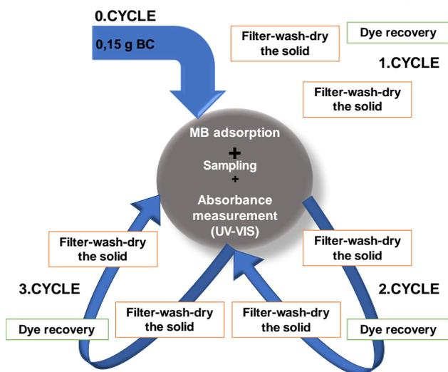
Figure 1: BC recovery and reuse experimental set.
