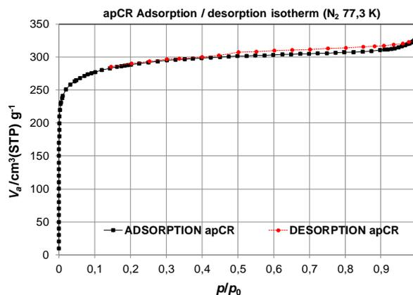
Figure 2b: apCR N<sub>2</sub> adsorption-desorption isotherms
