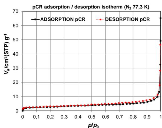
Figure 2a: pCR N<sub>2</sub> adsorption-desorption isotherms
