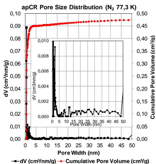
Figure 3b: apCR pore size distribution curves (NDFT)
