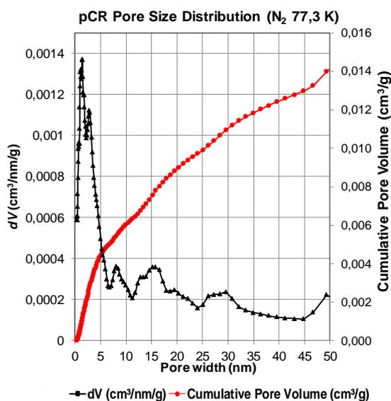
Figure 3a: pCR pore size distribution curves (NDFT)
