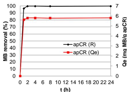
Figure 4: MB removal (R) and adsorption ratio (Qe) for apCR samples.
