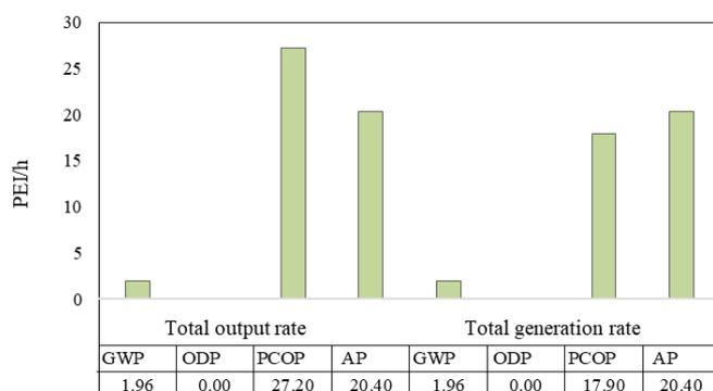
Figure 5. Atmospheric impacts of microalgae-based biodiesel production via in-situ transesterification.
