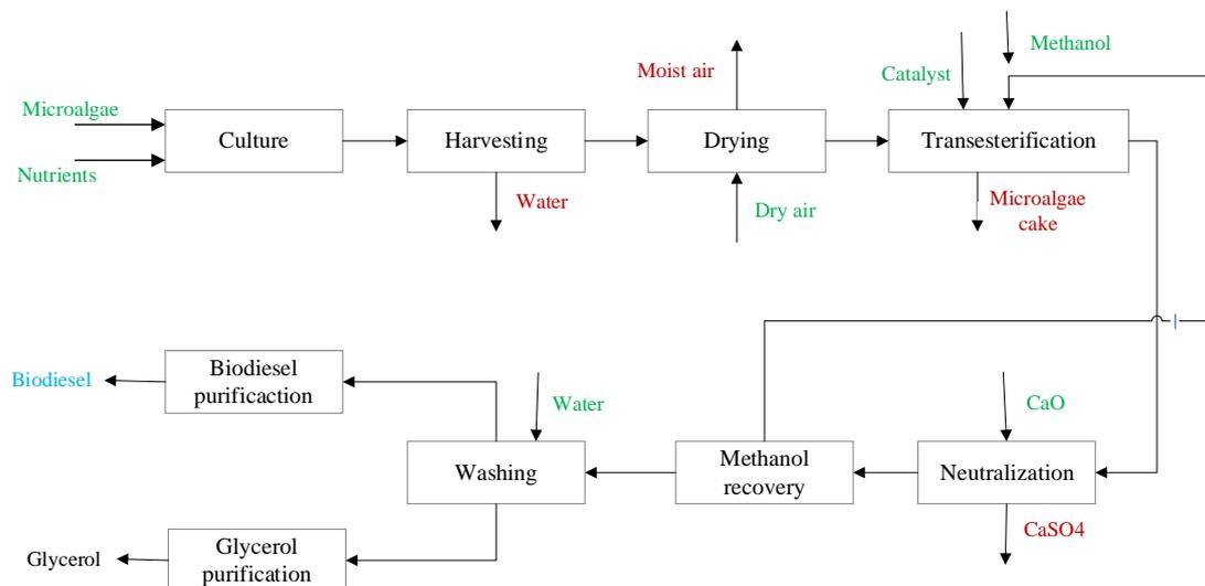
Figure 1. Block diagram of microalgae-based biodiesel production via in-situ transesterification
