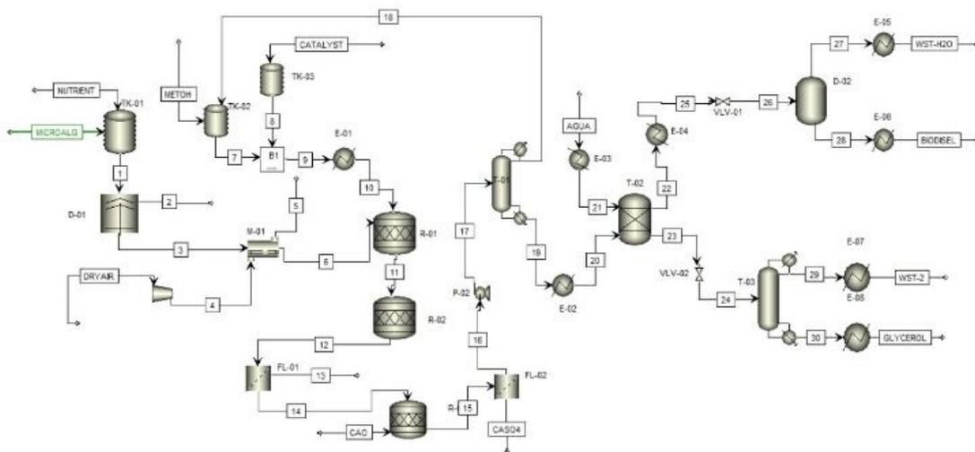
Figure 2. Simulation of microalgae-based biodiesel production via in-situ transesterification
