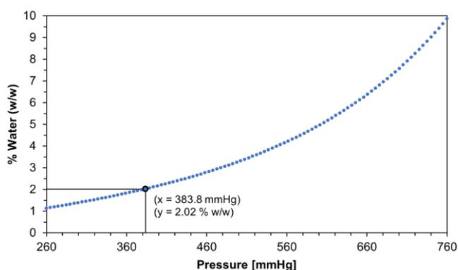
Figure 3: Parametric study of the flash vessel (V-101) pressure at a constant temperature of 115°C to analyse the water content in the dehydrated LA.
