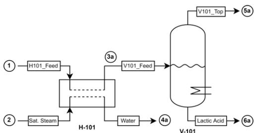
Figure 1: Flowsheet of the LA dehydration using a heat exchanger and a flash vessel.
