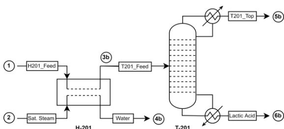
Figure 2: Flowsheet of the LA dehydration using a heat exchanger and a distillation column.
