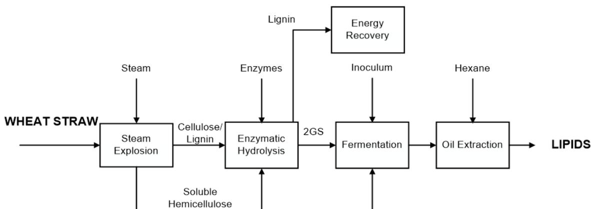
Figure 1: BFD for microbial oils production from lignocellulosic biomass
