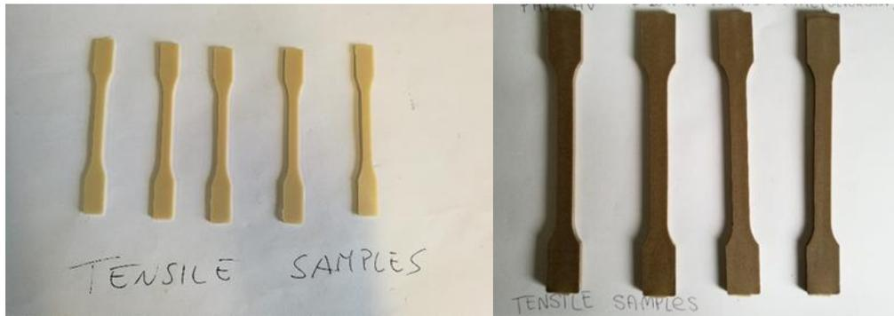
Figure 1: Tensile sample (PCA left, PCA with CS right)
