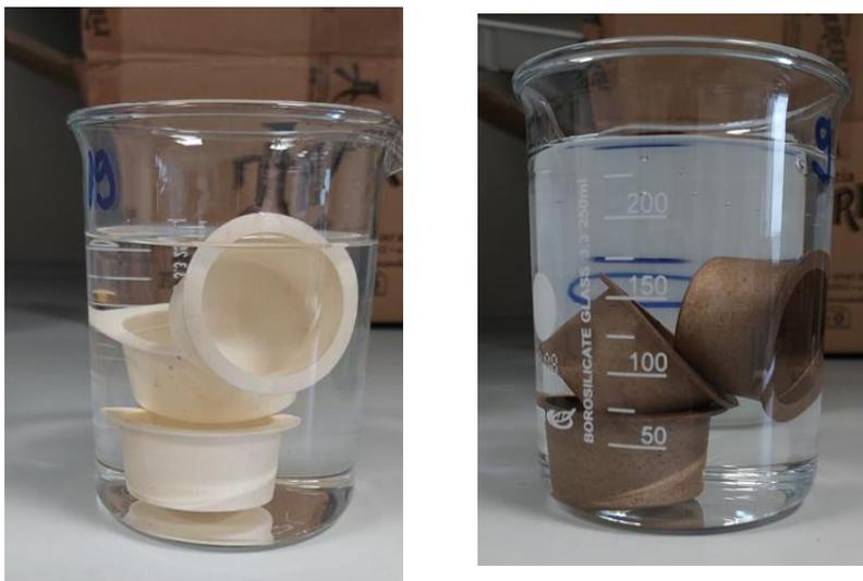
Figure 4: Migration test performed by immersion of injection moulded coffee capsules body (PCA left, PCA\_12.5 right)
