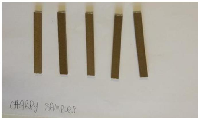
Figure 2: Charpy sample (PCA with CS)
