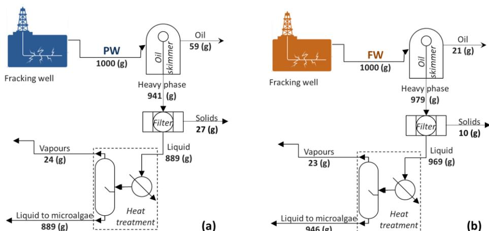
Figure 1. Mass balances around the unit operations used for the pre-treatment of PW (a) and FW (b)
