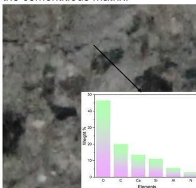
Figure 6: (a) Optical micrographs and EDX analysis of self-healed concrete with DNC-UF@SiO<sub>2</sub>.
