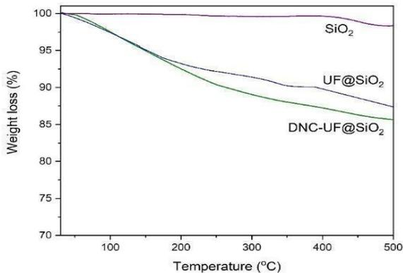
Figure 3: Thermogravimetric analysis of SiO<sub>2</sub> nanoparticles, UF-encapsulated SiO<sub>2</sub> (UF@SiO<sub>2</sub>), and DNC-UF encapsulated SiO<sub>2</sub> (DNC-UF@SiO<sub>2</sub>).
