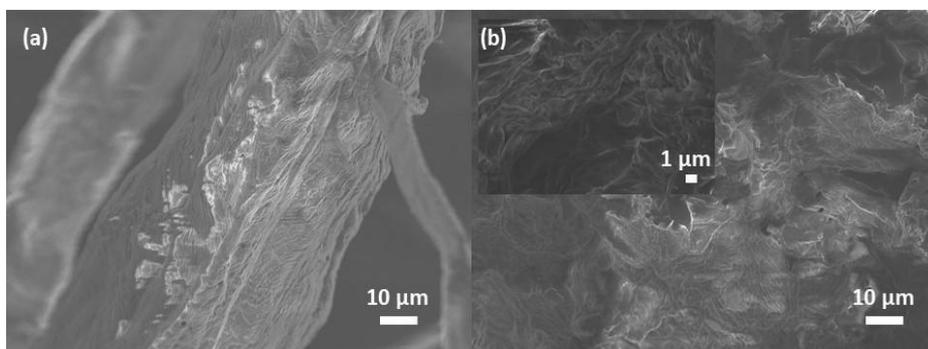
Figure 1: SEM micrographs of (a) extracted fiber and (b) nanocellulose from durian rinds.
