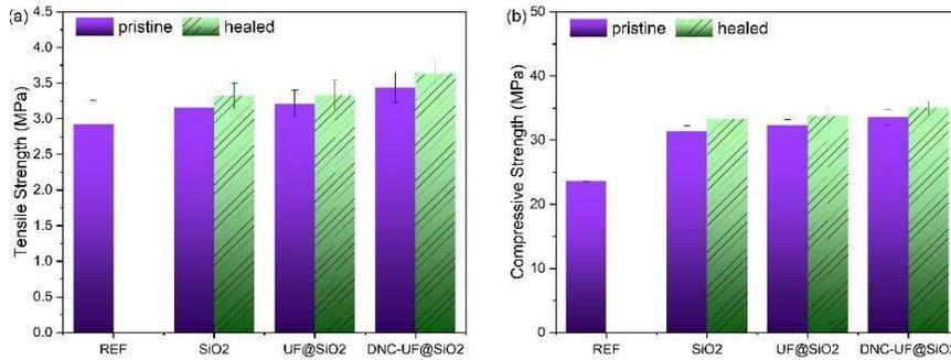
Figure 4: (a) Compressive and (b) tensile strength of pristine and healed concrete at 28 days.
