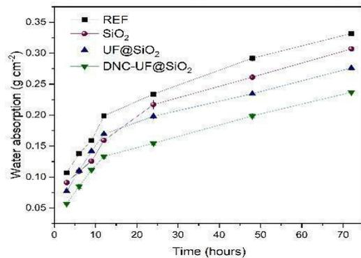
Figure 5: Water absorption by capillarity of cracked concrete samples after 28 days.
