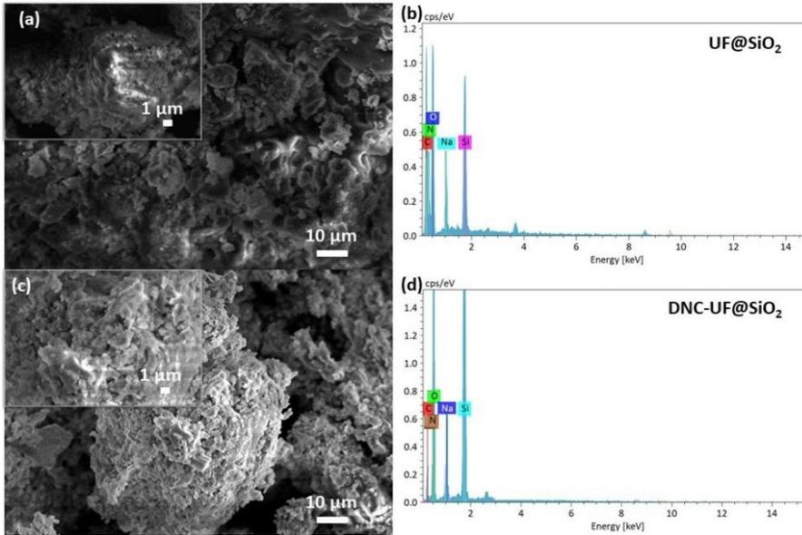
Figure 2: SEM micrographs and EDX analysis of (a, b) UF encapsulated SiO<sub>2</sub> (UF@SiO<sub>2</sub>), (c, d) DNC-UF encapsulated SiO<sub>2</sub> (DNC-UF@SiO<sub>2</sub>).
