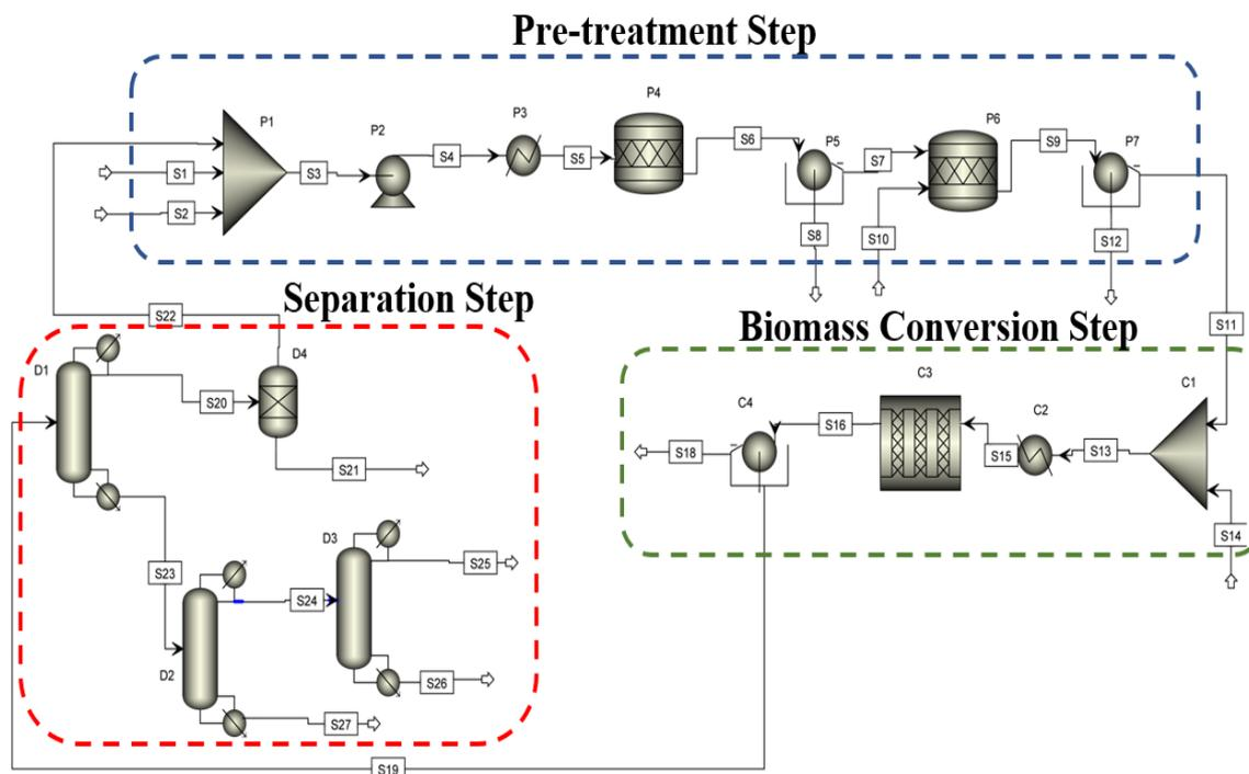
Figure 1: Process flow diagram of 5-hydroxymethylfurfural production using sugarcane bagasse as raw material.
