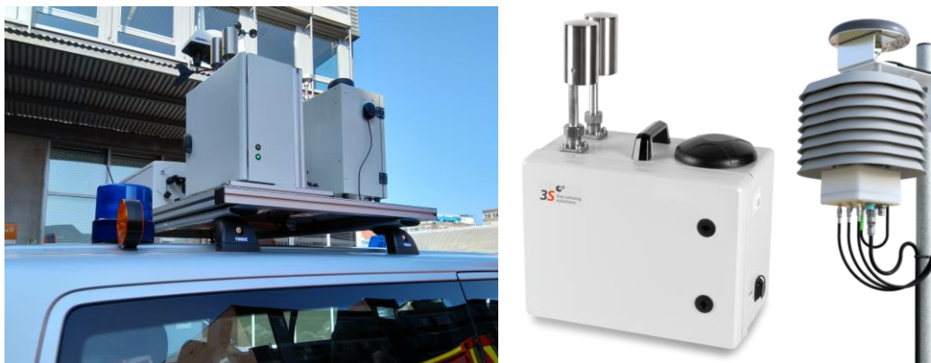
Figure 5: Mobile sensor devices mounted on a vehicle (left) and semi-stationary device (middle) for explorative use in temporary or establishing projects. Lightweight network node with diffusion access (right).
