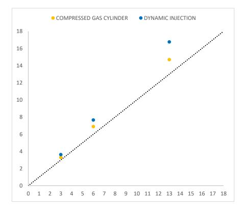
Figure 3. Dynamic injection vs known concentration gas cylinder at medium concentration - toluene
