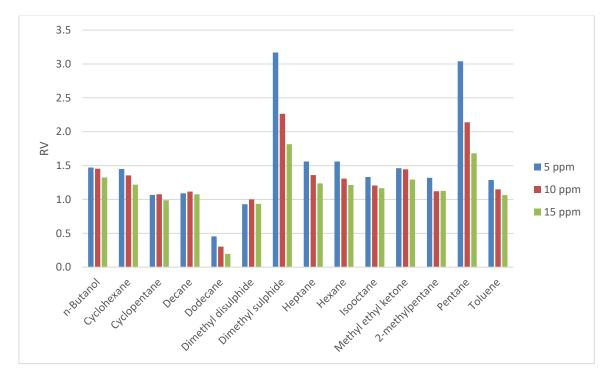
Figure 2. Ratio value (RV): measured values vs expected values
