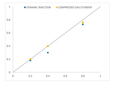
Figure 4. Dynamic injection vs known concentration gas cylinder at low concentration - toluene
