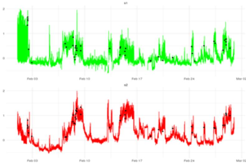
Figure 4: eNoses signals of s1 (green) and s2 (red) channels. Complaints are shown at the related timestamps (black dots).
