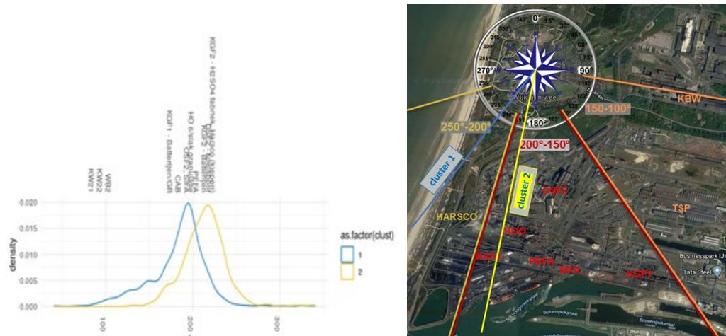
Figure 7: clusters 1 and 2 wind direction distribution (left) and peak wind directions with respect to TATA Steel plant installations (right).
