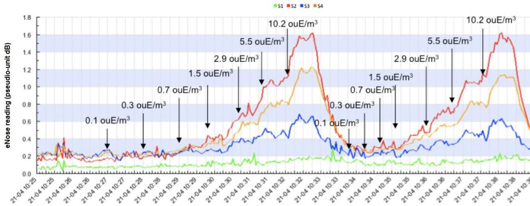
Figure 1: comparison between dynamic olfactometry and eNose readings for the TATA steel sinter plant odour.
