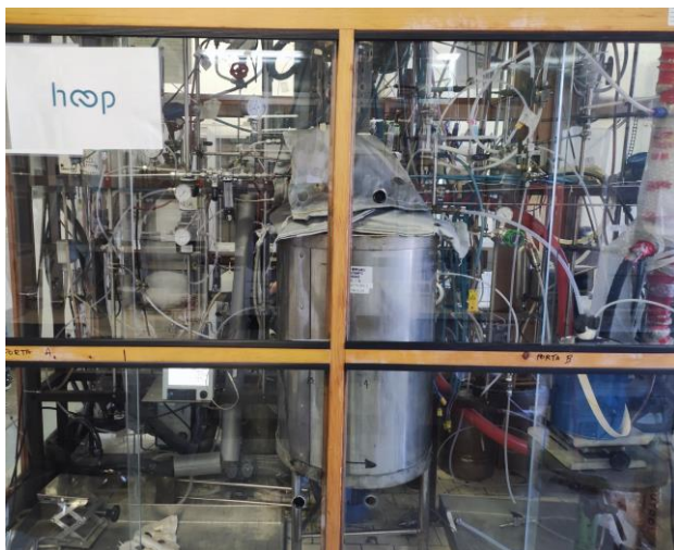
Figure 2. Hoop@ lab-scale pyrolysis reactor
