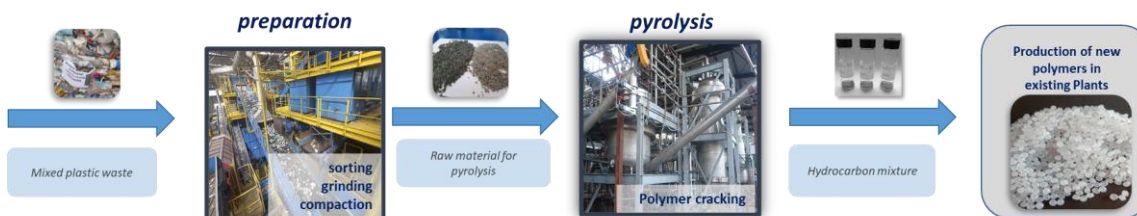
Figure 5. Chemical recycling via pyrolysis
