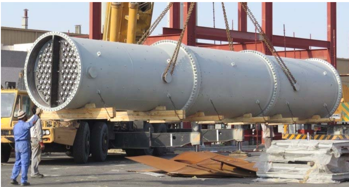
Figure 7: Cyclic distillation (dividing-wall) column prepared for transportation to be installed on a chemical site
