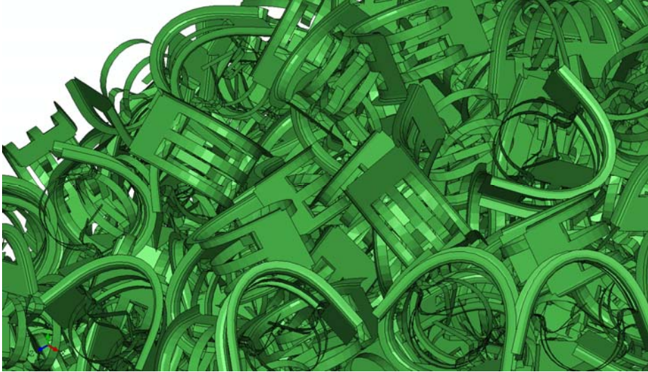
Figure 2: Output of Pasimodo ® for dumped I-Rings
