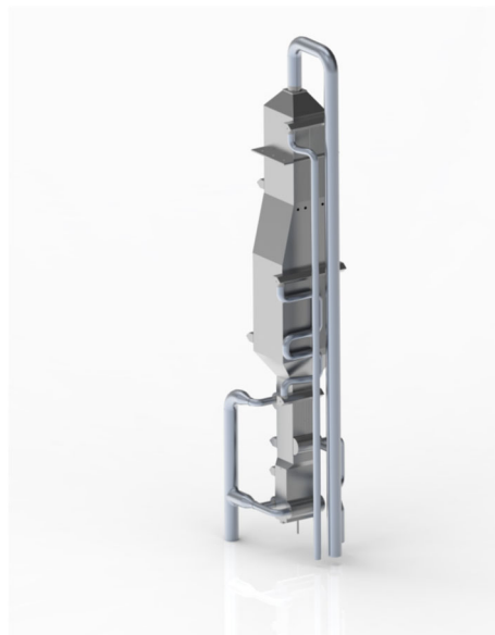
Figure 1. CAD model of the ammonia cracking reactor for 25 kg/h ammonia feed
