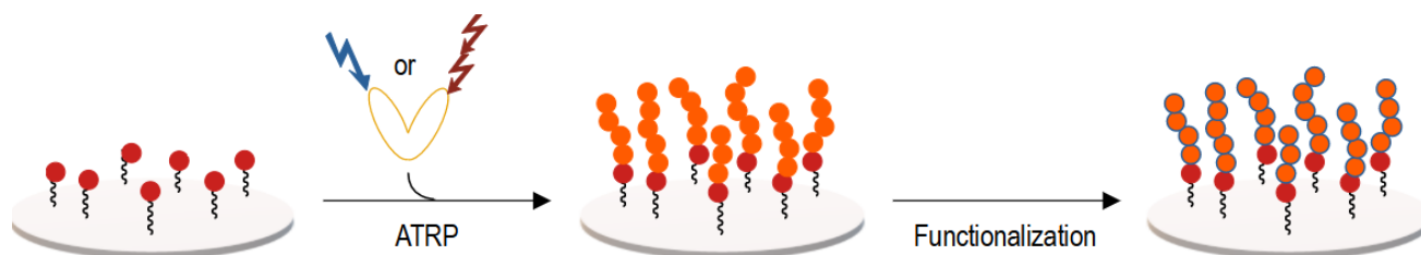
Figure 1 - Surface functionalization by photoinduced Surface Initiated ATRP.
