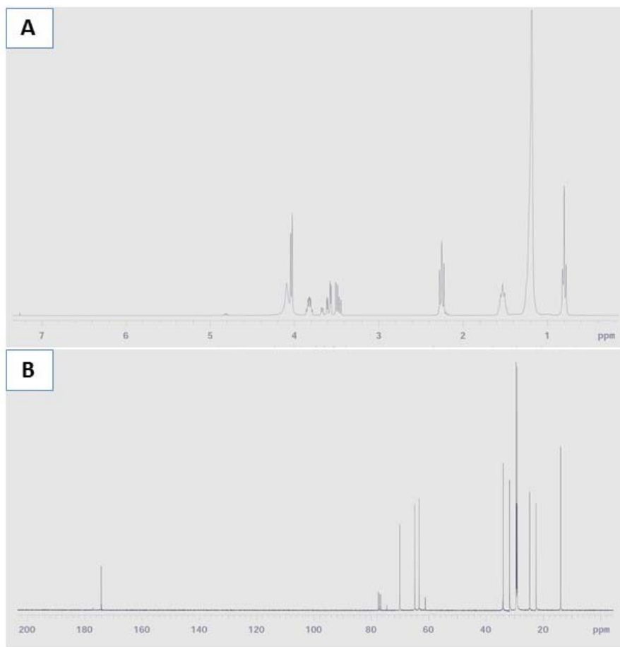
Figure 3: 1 H NMR (A) and 13 C NMR (B) spectra of the sodium 9,10-dihydroxy octadecanoate (sodium salt of hydroxylated oleic acid)
