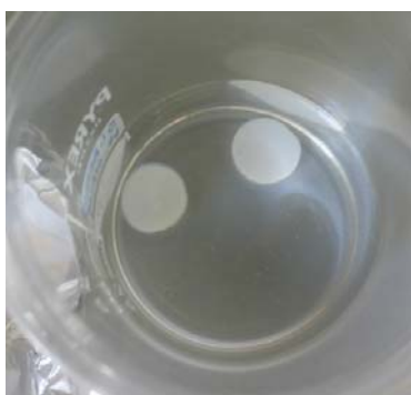
Figure 1: kefir scaffolds prepared via TIPS.
